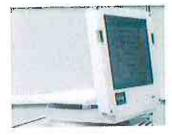
Dialog\* Evolution has a large, high resolution rotating, flat touch screen that provides a clear, highly visible user interface. The flat screen makes space available for the removeable tray behind the screen.
